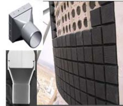
Ceramic honeycombs SOLAIR receiver (DLR), 2004.
