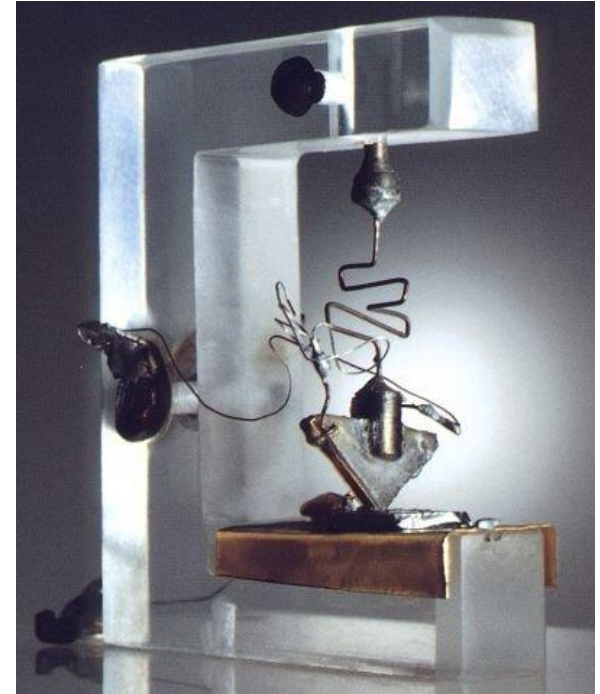
Ge used in the first transistor (1947, Shockley, Bardeen, Brattain)
